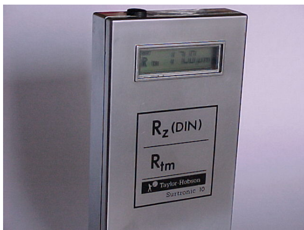
Picture 4: Measuring instrument for the determination of roughness
